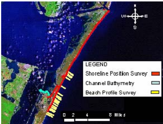
Figure 12. Shoreline position survey (red), channel hydrographic (green) and beach profile survey (yellow) data coverage.
